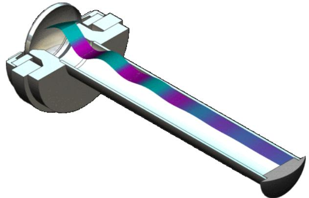
The image above shows the behaviour of the tweeter vent. Rear radiation from the dome travels down the duct and is gently absorbed in the acoustic damping material.
