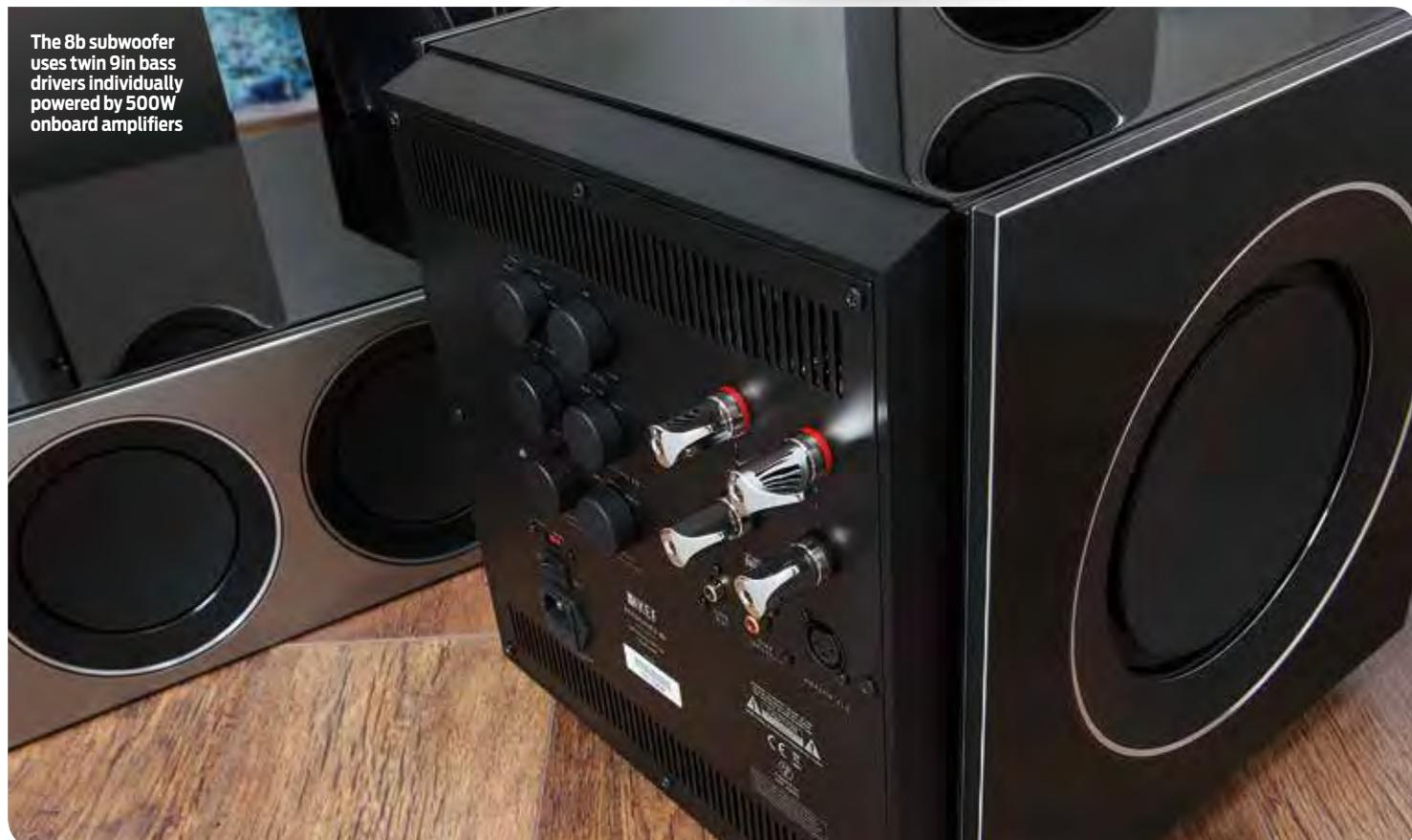
The 8b subwoofer uses twin 9in bass drivers individually powered by 500W onboard amplifiers
