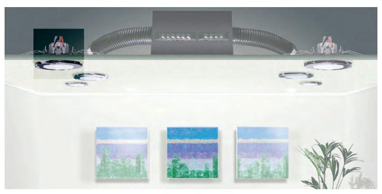
Loudspeaker installations don't come more discreet than the Ci50 Soundlight System. A full bandwidth sound system consisting of four satellite speakers and a twin-ported subwoofer, the only visible components are designed to be virtually indistinguishable from a standard 50mm low voltage light fitting once installed. The subwoofer itself is hidden out of sight in the ceiling void, with a 100mm (4") dual
